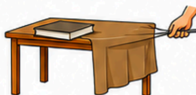
When a cloth is pulled quickly, the book remains in place due to inertia.
