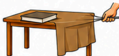
When a cloth is pulled quickly, the book remains in place due to inertia.
